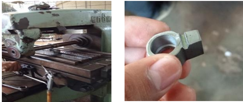
Gambar 21. Proses Milling Horizontal
