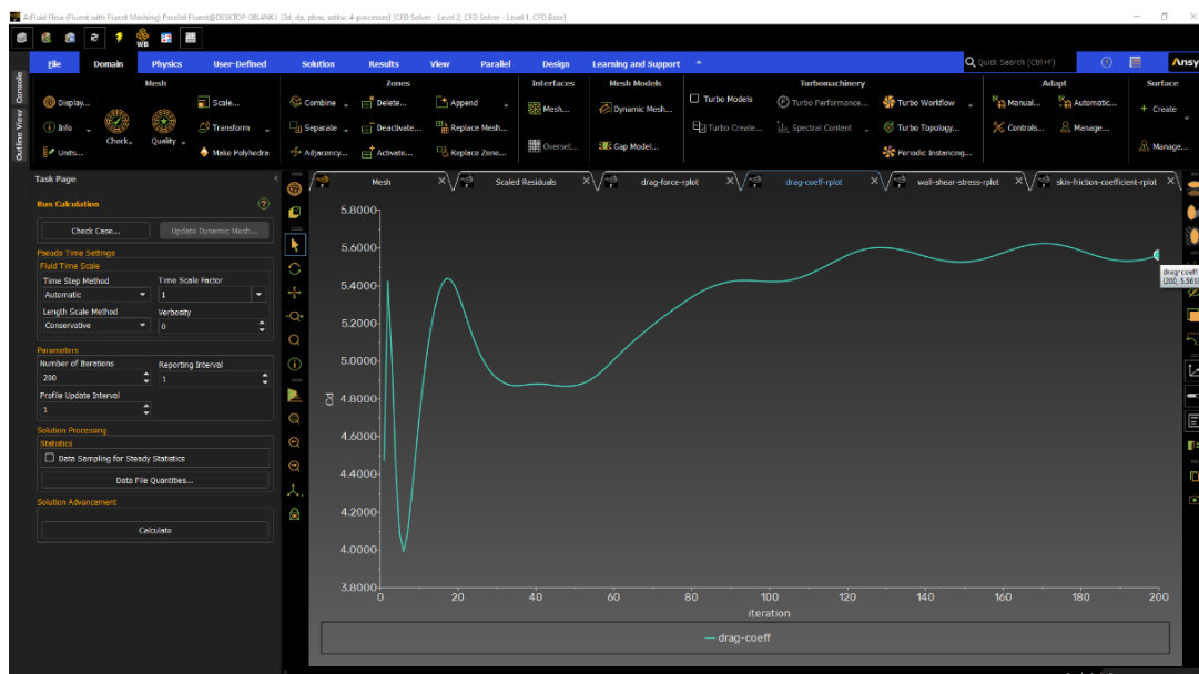
Gambar 3. Monitoring Drag Force dan Drag Coefficient
