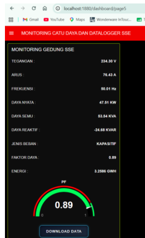
Gambar 2. Antarmuka Dashboard Monitoring Real-Time Berbasis Node-RED
